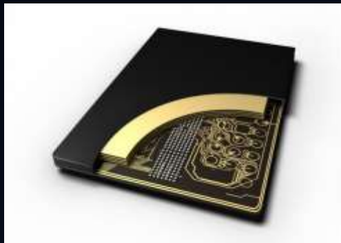
Figure 6.3 RDIMM Chip using 3D TSV packaging technology [14]
