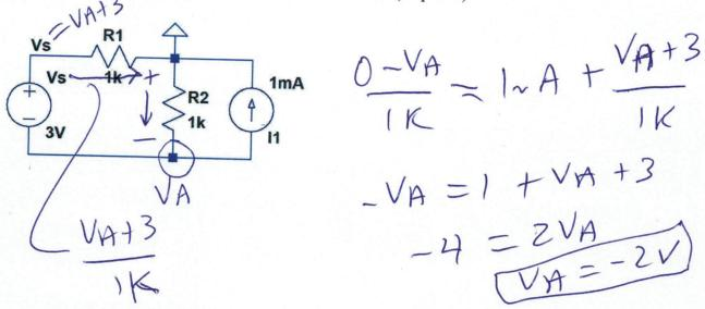
3. Find the voltage Vx in the circuit seen below. Then find the Thevenin equivalent circuit, with R2 removed, at the terminals marked by dots. Show that your Thevenin circuit is correct by comparing the value you calculated for Vx to the one you get when you put R2 across the terminals of your Thevenin equivalent. (20 points) 1.5k
