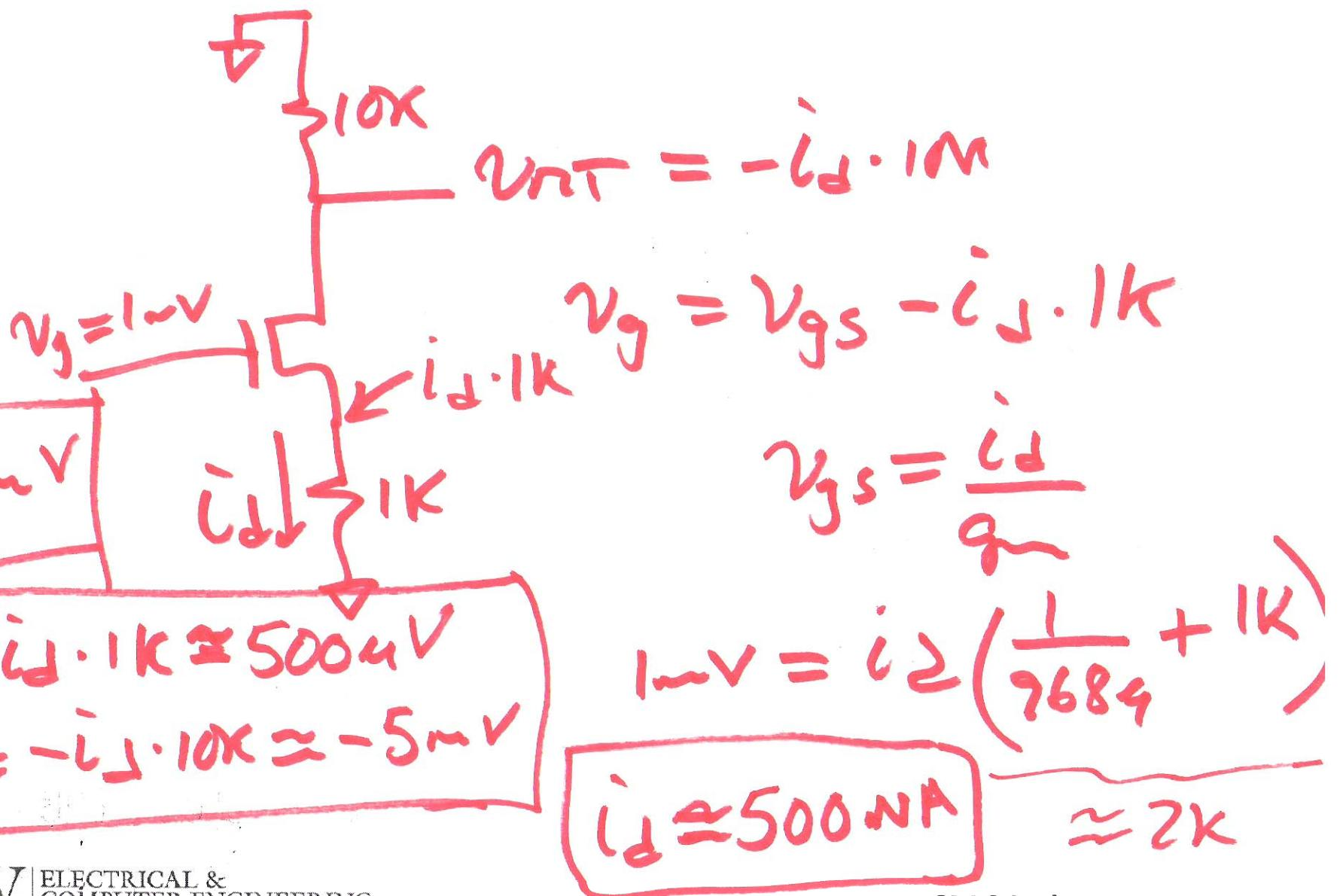
3. Calculate the AC and DC voltages on the gate, drain, and source of the PMOS transistor in the following circuit. Show your work for credit. (20 points)
