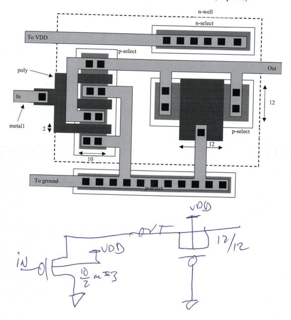
the sheet resistance is 1k/square. Make sure to label each of the layers in your layout. Sketch the cross-sectional view of your layout. Explain what the hires layer does during the fabrication process. (20 points) hi-res blocks poly2 from being depet 6 al > p2 / (elec)
