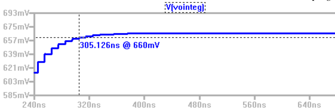
Figure 6: Non-ideal op-amp with input parasitic capacitor
