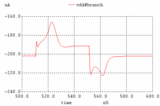
Fig 8 Current pulled from VDD for VDD=1.2V
