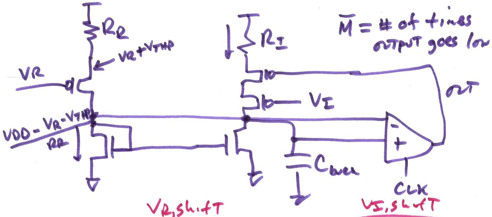
$$\frac{V_{DD} - V_R - V_{THP}}{R_E} = \frac{V_{DD} - V_I - V_{THP}}{R_E \cdot \frac{\bar{M}}{2}}$$
