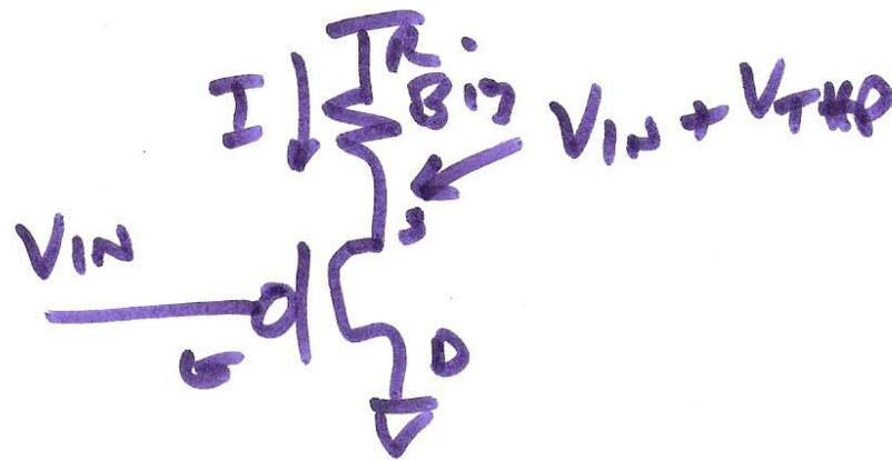
$$I = \frac{V_{DD} - (V_{IN} + V_{THP})}{R_{Big}}$$
