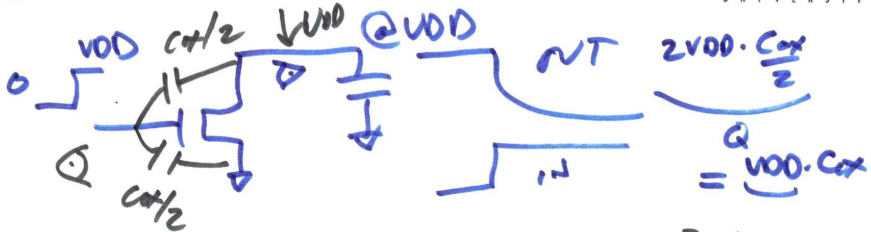
$$\frac{3}{2} C_{ox} = \frac{3}{2} C_{ox}' \cdot L \cdot W = \frac{3}{2} \frac{\epsilon_{ox}}{t_{ox}} \cdot L \cdot W$$
