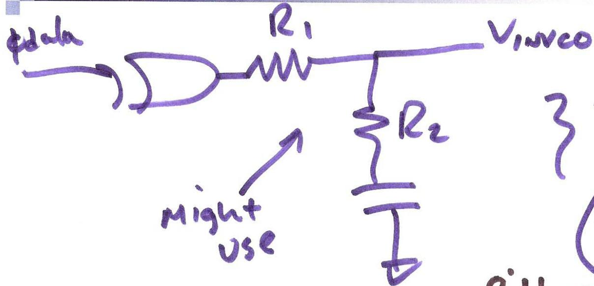
$$\omega_n = \frac{1}{2} \sqrt{\frac{K_p K_{vco}}{N(R_1 + R_2)C}}$$
