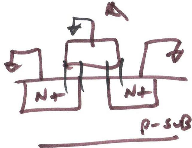
$$C_{in} = C_{GDO} \cdot W + C_{GSO} \cdot W$$
