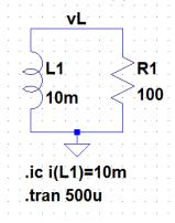
2. For the following circuit determine, and plot, the current in the inductor and the voltage across the inductor. Show your work (be very clear). Also plot the energy stored in the inductor against time. Verify all three plots using LTspice.
