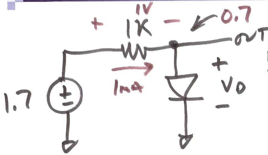
$$r_d = \frac{25mV}{1mA} = \frac{V_T}{I_{diode}} = 25\Omega$$
