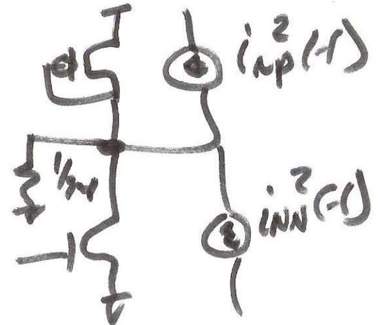
$$V_{noise}^2(f) = \left( \frac{1}{g_m} \right) \cdot (2.4 + 2.67) \cdot 10^{-24} \frac{\text{A}^2}{\text{Hz}}$$
