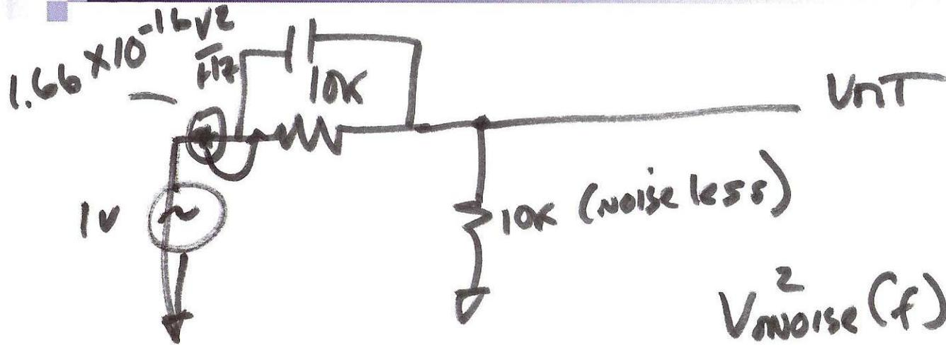
$$V_{\text{noise}}^2(f) = 1.66 \times 10^{-16} \cdot \left( \frac{10\text{k}}{10\text{k} + 10\text{k}} \right)^2$$
