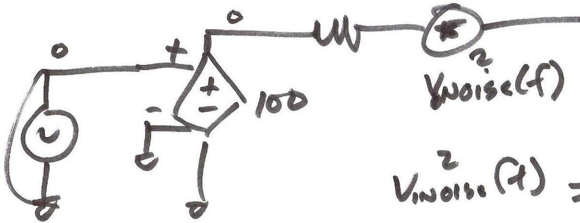
$$V_{\text{noise}}^2(f) = 1.66 \times 10^{-16} \frac{\text{V}^2}{\text{Hz}}$$
