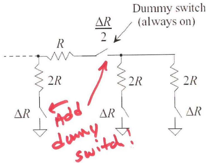
Figure 29.6 Use of dummy switches to offset switch resistance.
