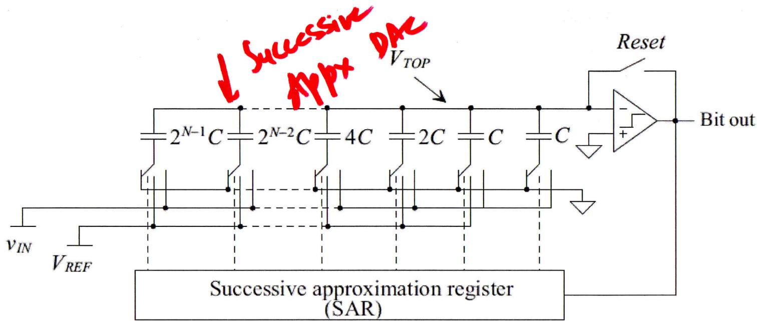
Figure 29.39 A charge redistribution ADC using a binary-weighted capacitor array DAC.
