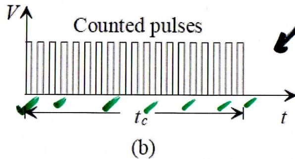
Figure 29.33 Single-slope ADC timing diagrams for (a) the comparator inputs and outputs and (b) the resulting counted pulses.
