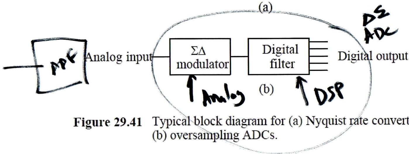
Figure 29.41 Typical block diagram for (a) Nyquist rate converters and (b) oversampling ADCs.
