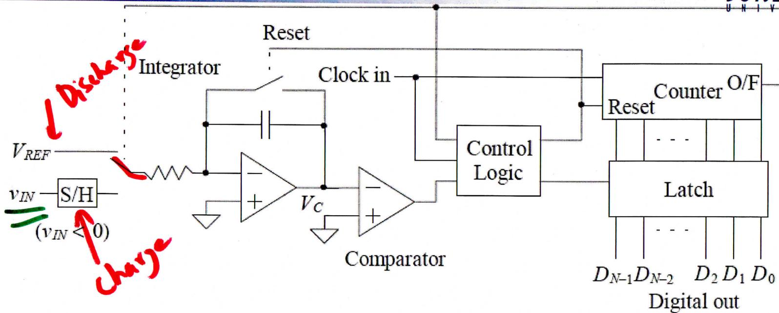
Figure 29.34 Block diagram of a dual-slope ADC.
