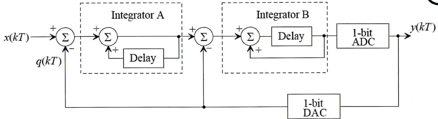
Figure 29.49 A second-order, sigma-delta modulator.
