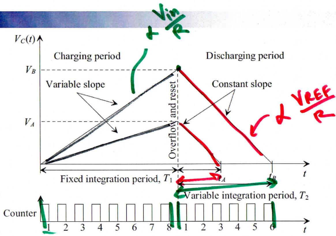
Figure 29.35 Integration periods and counter output for two separate samples of a 3-bit dual-slope ADC.
