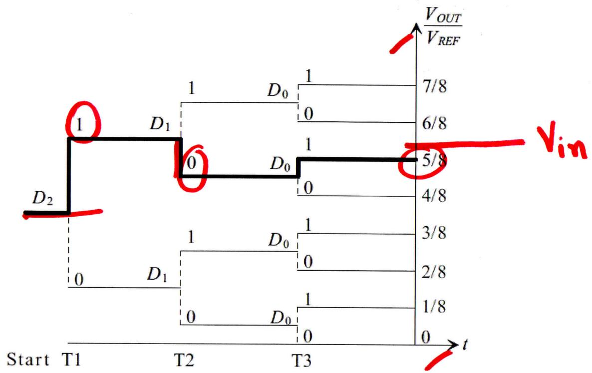
Figure 29.37 Binary search performed by a 3-bit successive approximation ADC for  $D=101$ .
