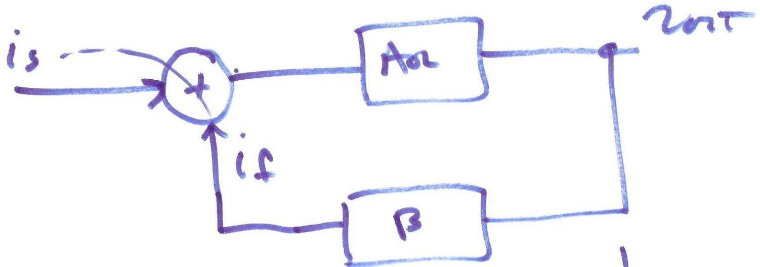
$$i_s = \frac{v_{out}}{\beta} = -i_f \Rightarrow \beta = -\frac{1}{R_2}$$
