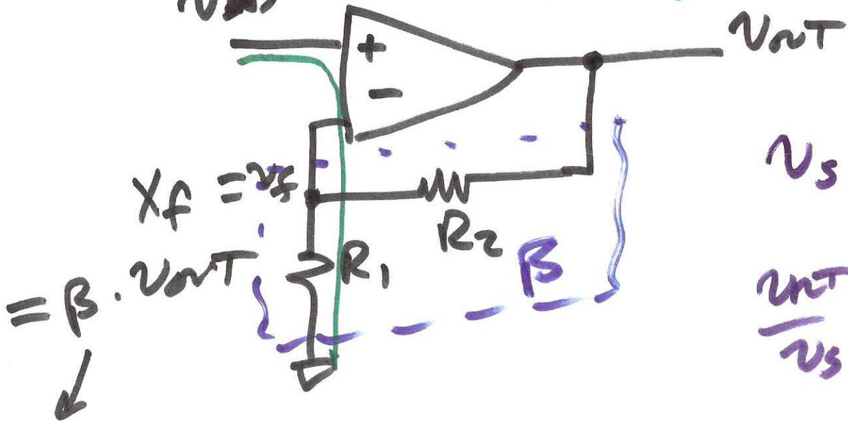
$$V_s = V_{out} \cdot \frac{R_1}{R_1 + R_2}$$
