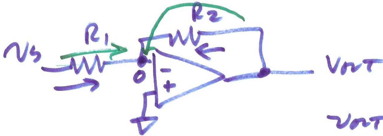
$$\frac{v_{OUT}}{v_s} = -\frac{R_2}{R_1}$$
