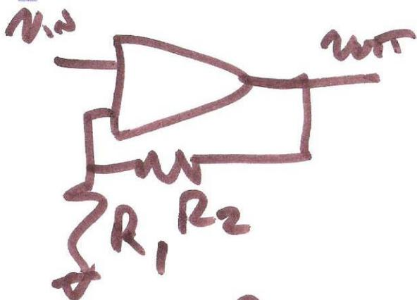
$$\beta = \frac{R_1}{R_1 + R_2}$$
