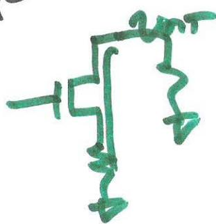
INPUT SERIES - VOLTAGE - SHUNT
