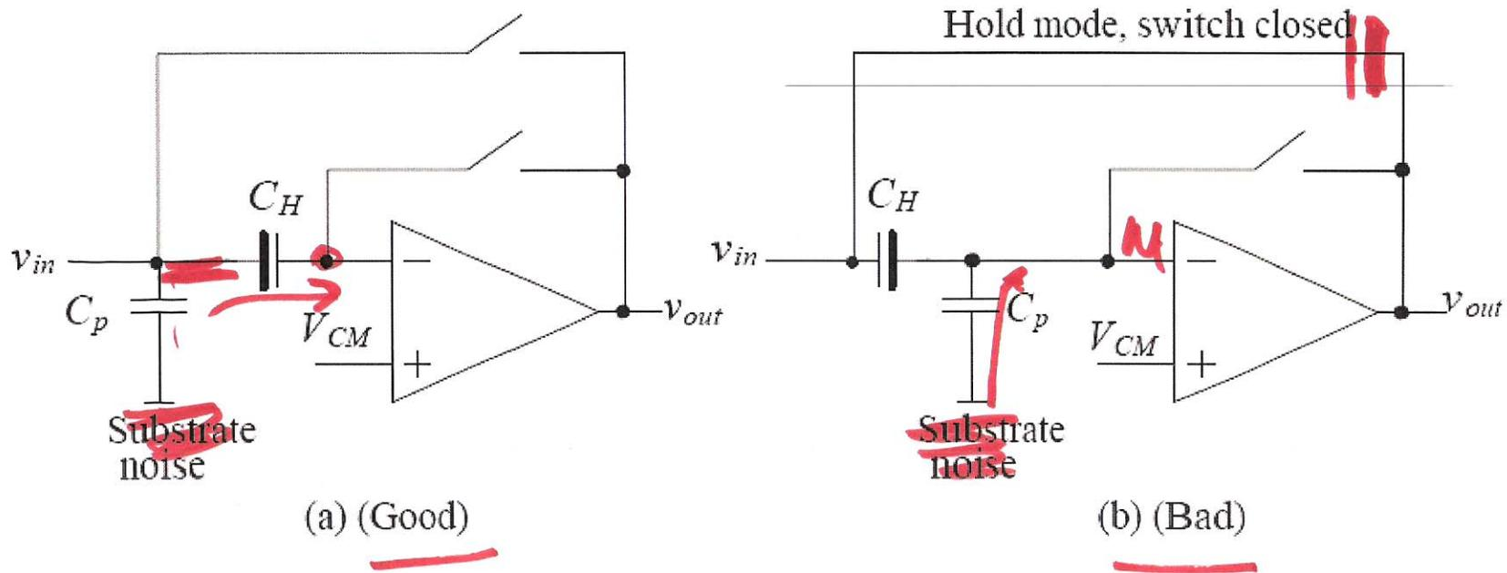
Figure 25.16 Explanation for connecting the bottom plate of the capacitor to the input.
