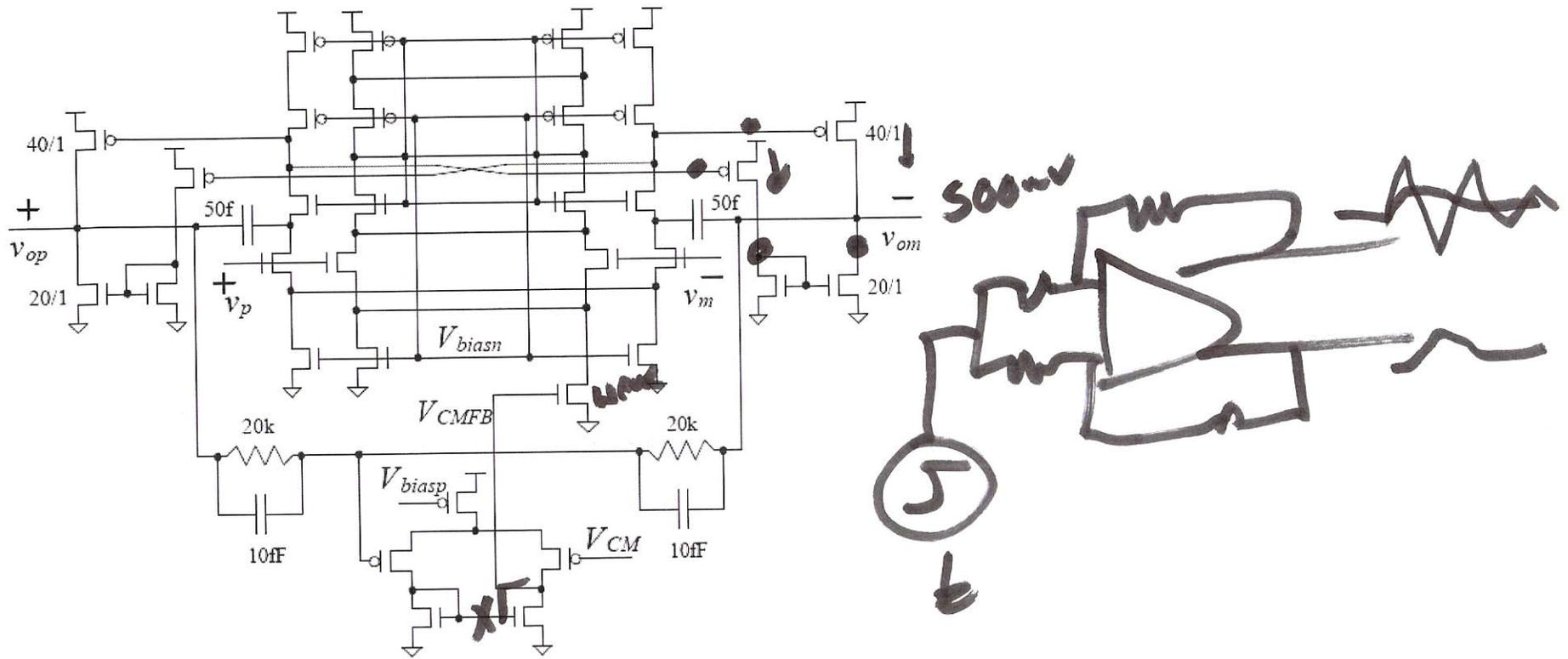
Figure 26.29 Complete schematic of op-amp with CMFB.
