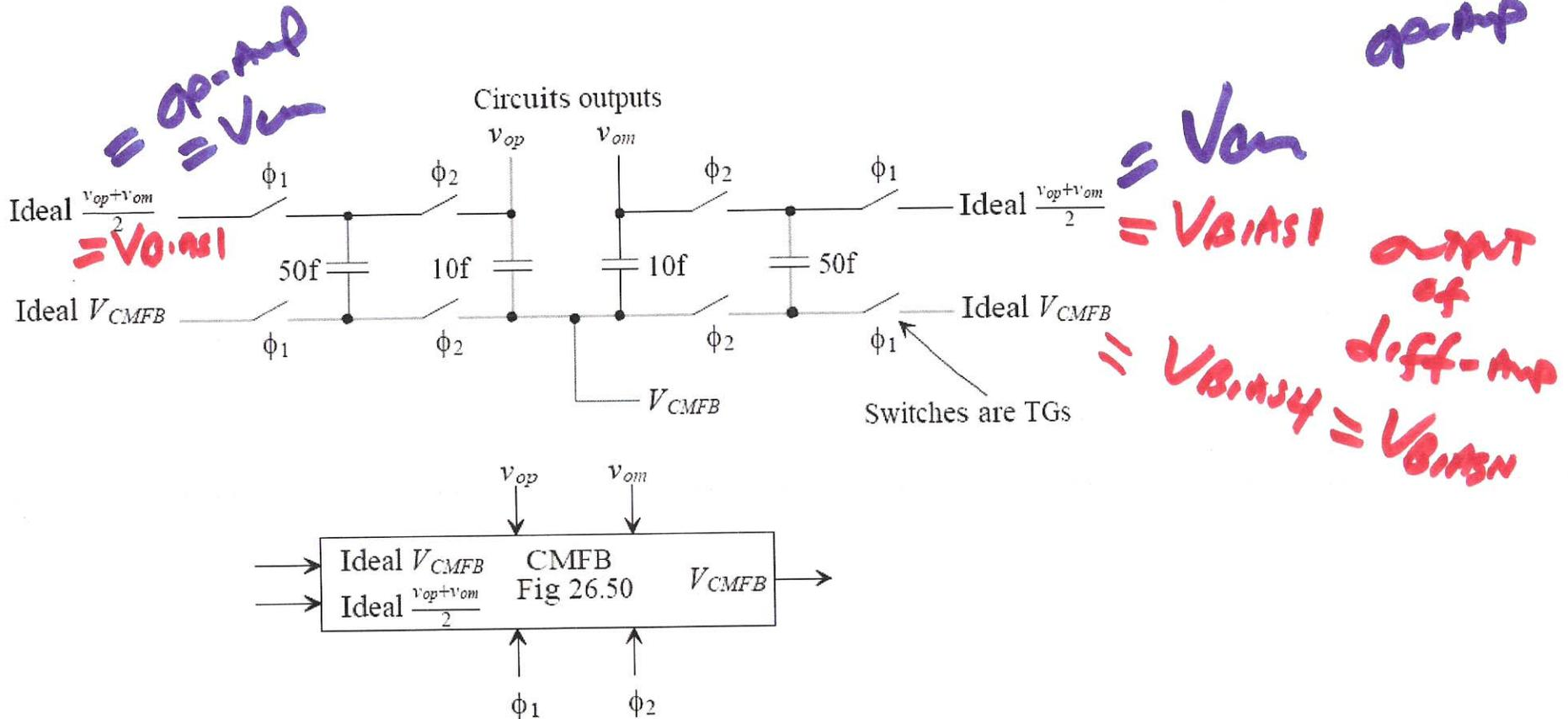
Figure 26.50 A switched-capacitor CMFB circuit (see Fig. 26.16).
