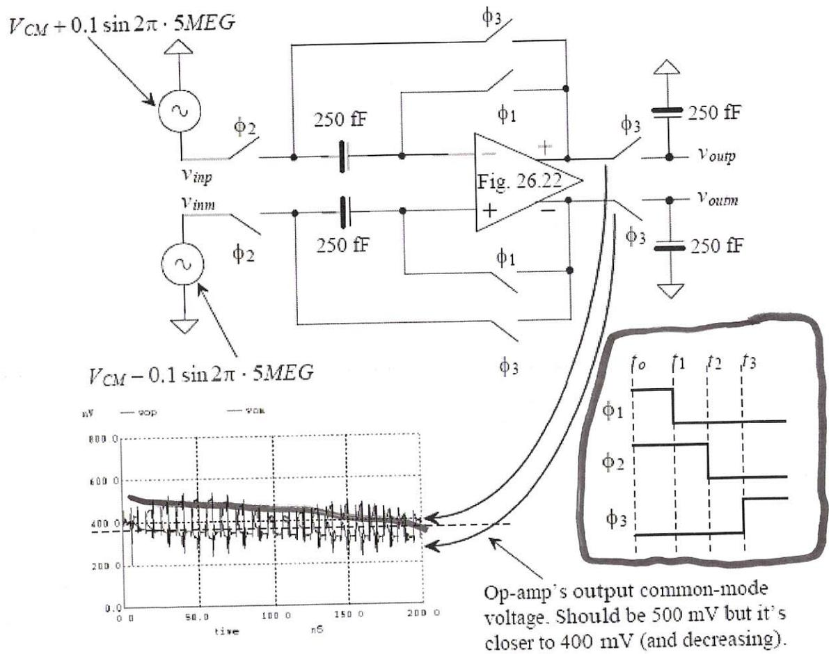
Figure 26.25 A sample-and-hold circuit. Notice how the output common-mode voltage is wandering.
