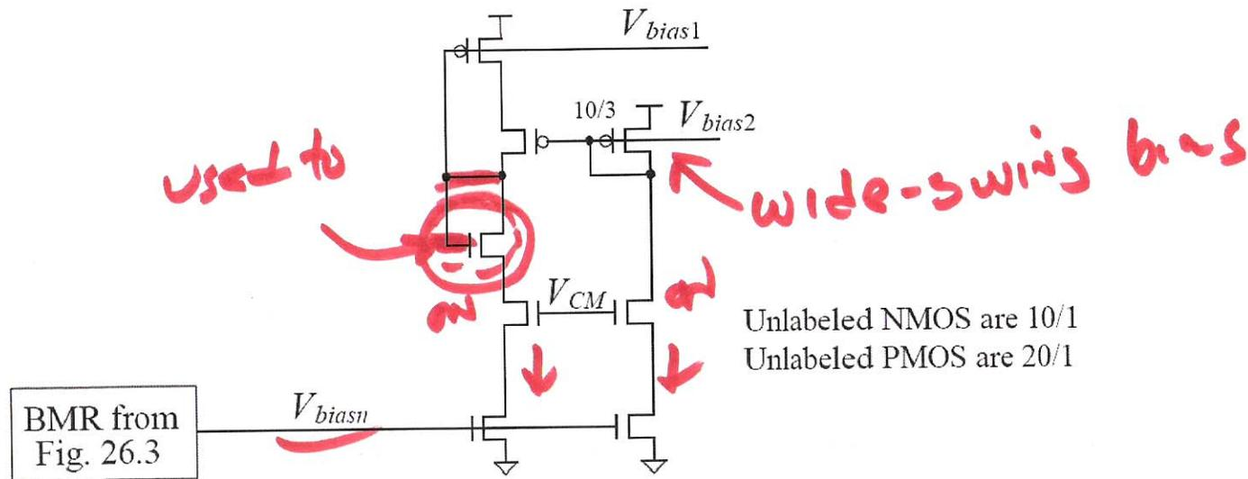
Figure 26.52 Biasing circuit for the op-amp developed in this section.
