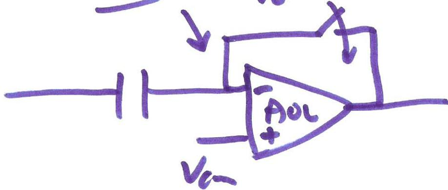
$$V_{OUT} = A_{OL}(V_+ - V_-)$$
