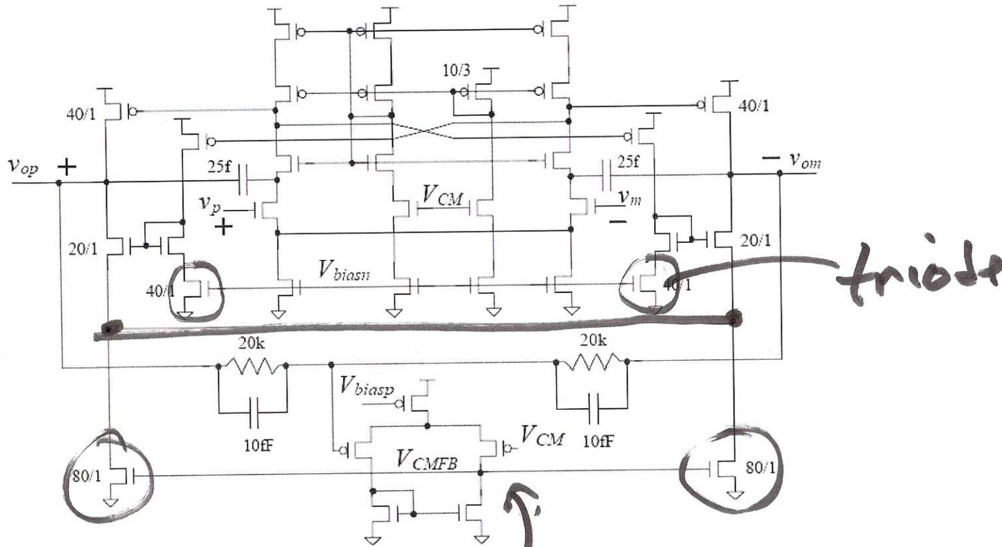
Figure 26.43 Providing CMFB through just the output buffer. Using an amplifier with triode-operating MOSFETs for CMFB (good).
