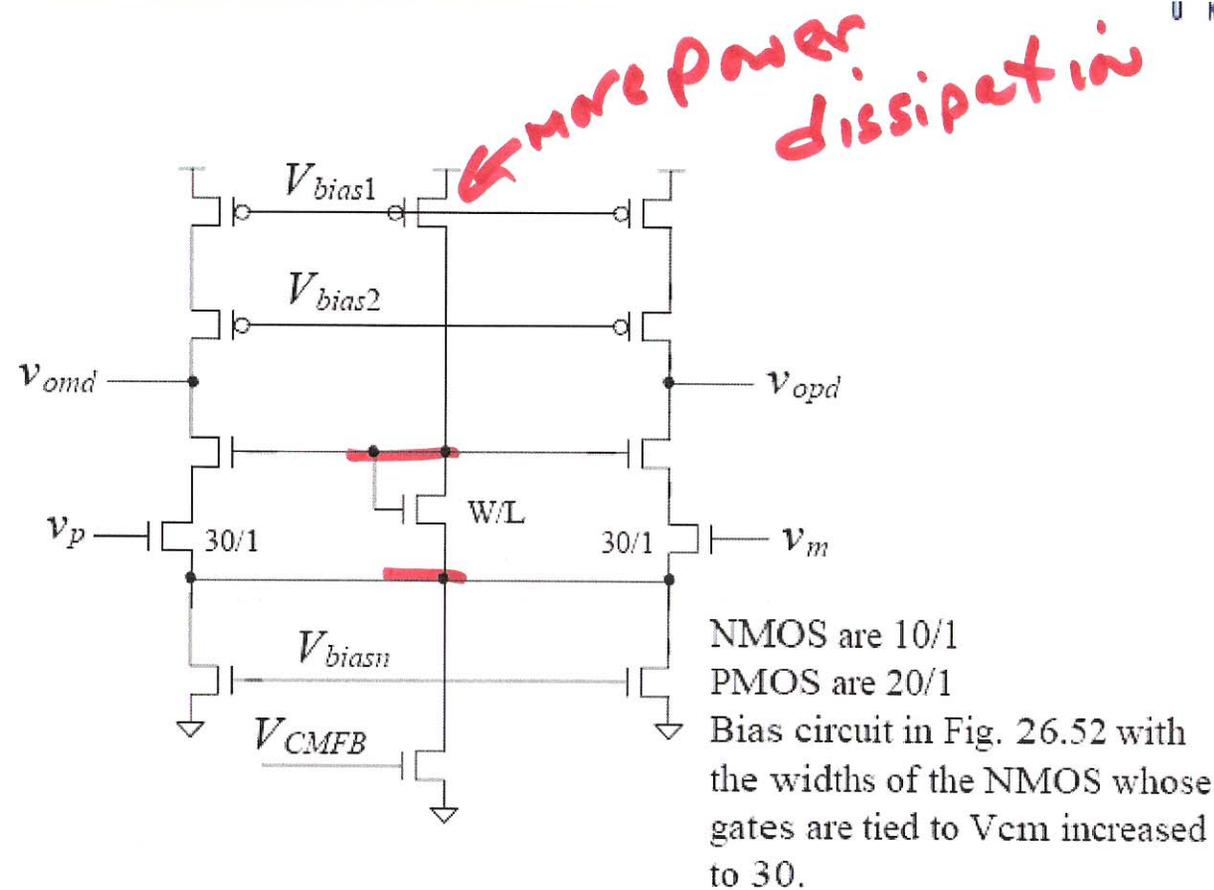
Figure 26.63 Modifying the diff-amp seen in Fig. 26.53 for wider swing operation.
