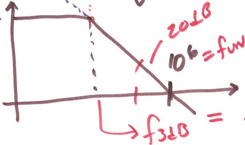
$$f_{3dB} = \frac{f_{UN}}{A_{voc}} = \frac{10^6}{10^3} = 10^3 \text{ Hz}$$
