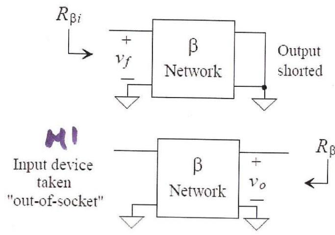
Figure 31.15 Determining the loading due to the feedback network for a series-shunt amplifier.
