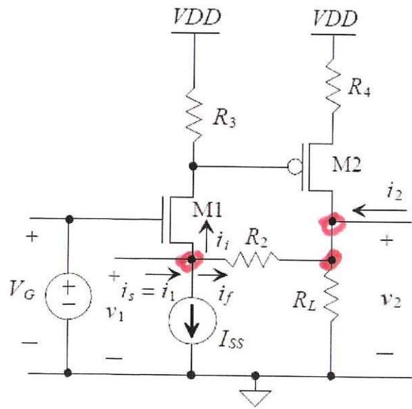
Figure 31.19 Shunt-shunt feedback amplifier.
