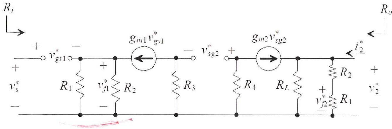
Figure 31.16 Open-loop small-signal model of Fig. 31.13.
