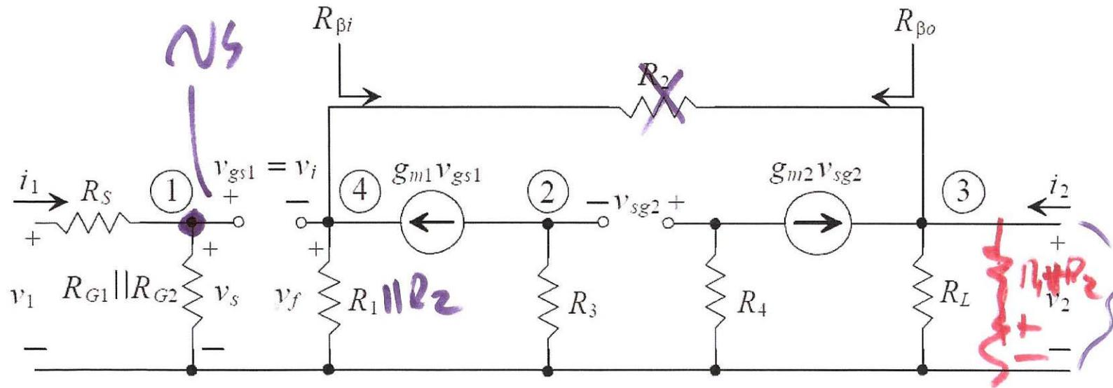
Figure 31.14 Closed-loop small-signal model of Fig. 31.13.
