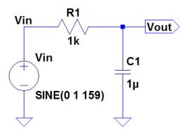
4. Determine the magnitude, |Vout/Vin|, and phase, Angle(Vout/Vin), responses of the circuit in problem 3. Verify your equations using a .ac (ac analysis). 3 points for hand calculations and 2 points for netlist and LTspice verification.
