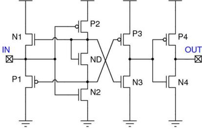
Figure 5: Schematic view of the current comparator.
