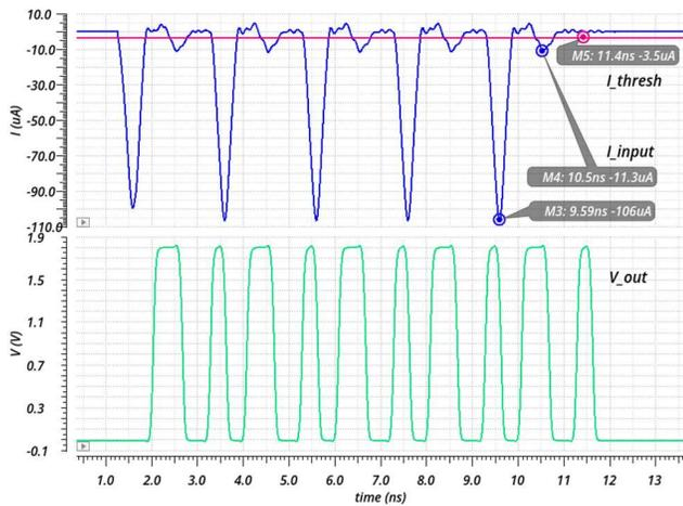
Figure 8: Response to alternating train of 10- $\mu$ A and 105- $\mu$ A pulses at 1-GHz.
