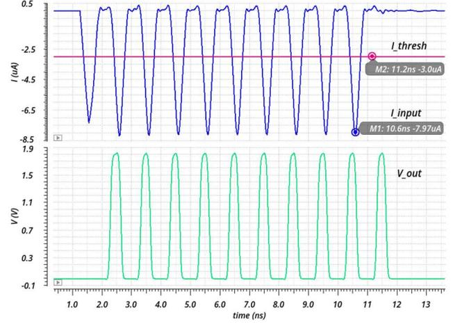
Figure 7: Response to train of 8-uA pulses at 1-GHz.
