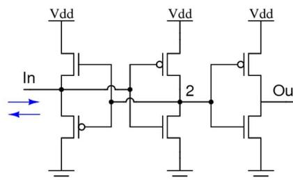
Figure 1: Schematic view of current comparator from [3].
