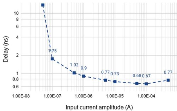
Figure 9: Plot of delay time as a function of input current amplitude.
