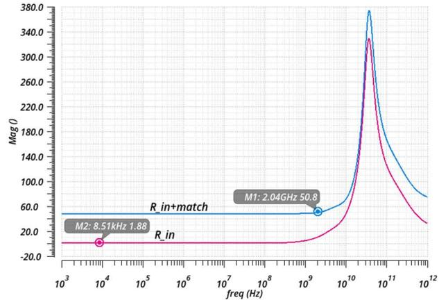
Figure 4: Simulation plot of input impedance.
