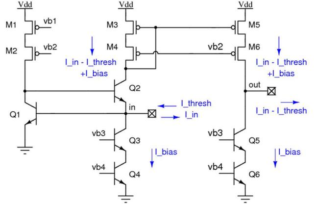
Figure 3: Current buffer stage with annotated currents. A bias of 250- $\mu$ A was used to bias each of the circuit branches.
