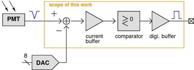
Figure 2: Block diagram of the proposed design.
