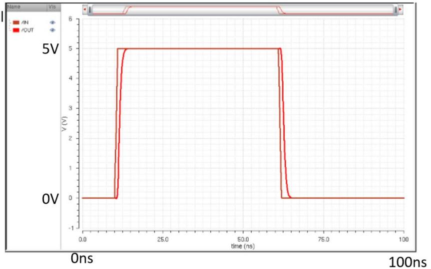
This simulation shows that the buffer can drive a 5pF load.
