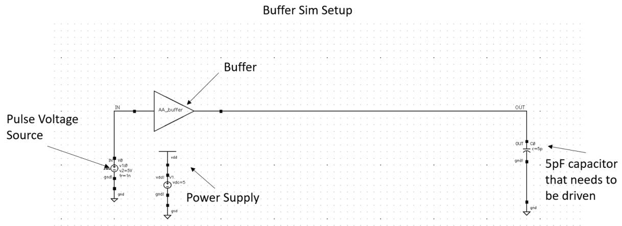
*Figure 32 - Buffer Simulation Schematics*
