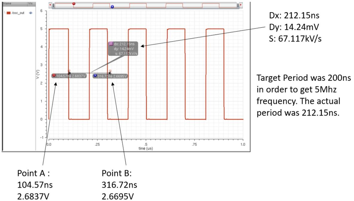
*Figure 17 - Ring Oscillator Simulation*
