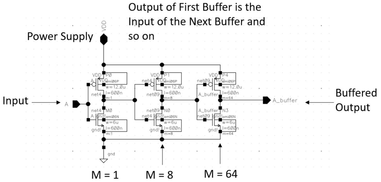
Notice that the M value goes up by \* 8. By using this method, it cuts down on schematic space. It is better than putting over 73 inverters
