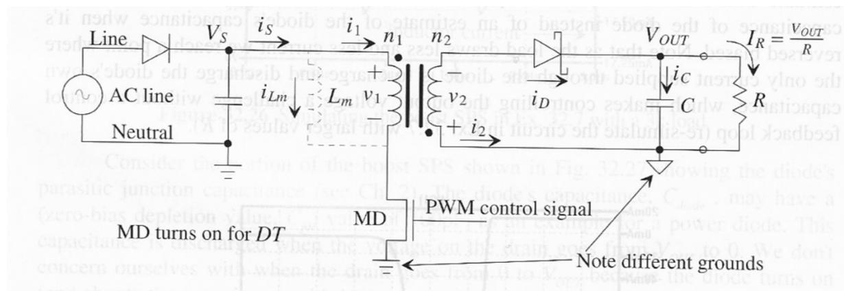
Figure 44 – Flyback SPS [1, Fig 32.29, p. 1200]
