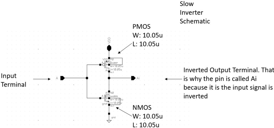
Figure 18 - Slow Inverter Schematic
