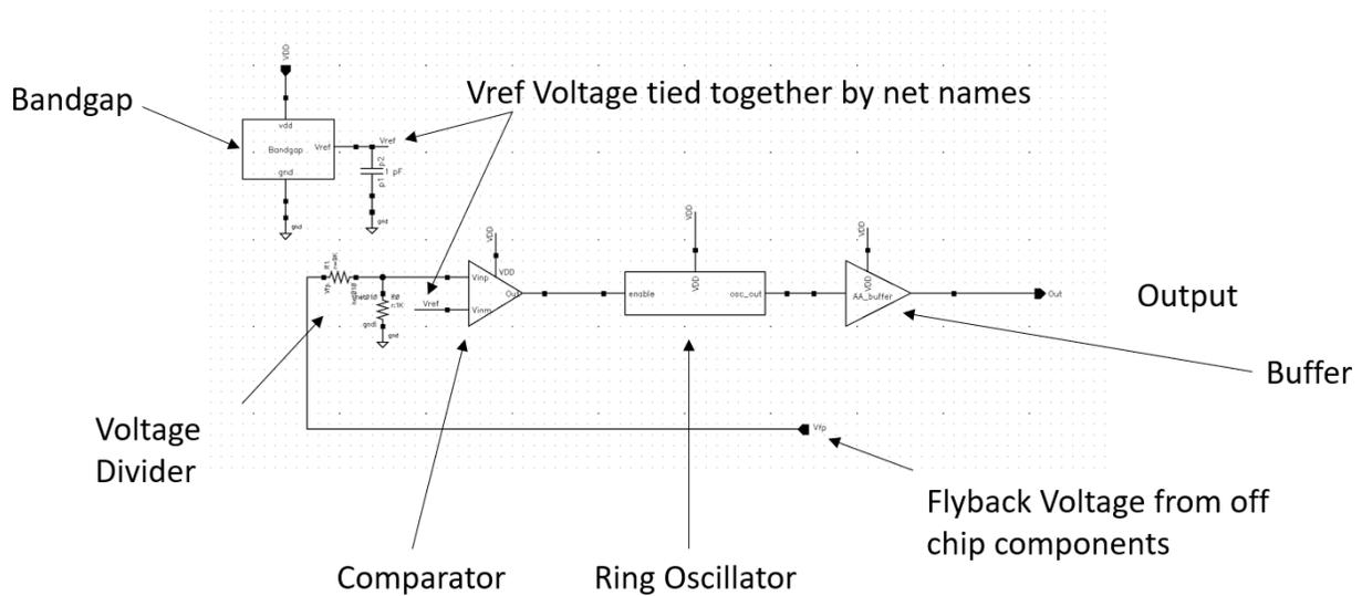
*Figure 41 - Top Level Schematic of the Controller Chip*
