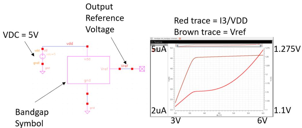
Figure 4 - Bandgap Response to Varying VDD Voltages
