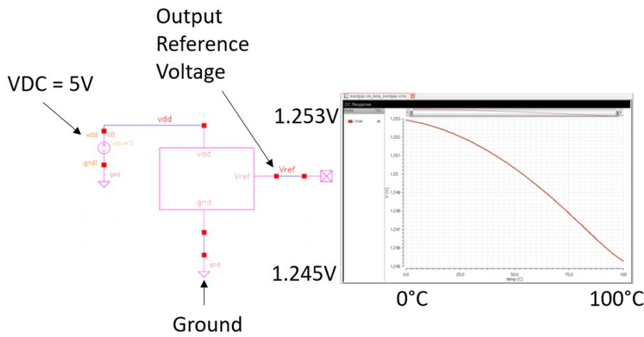
Figure 5 - Bandgap Response to Temperature
