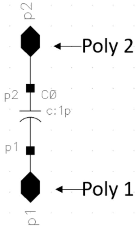
Figure 38 - 1pF Poly-Poly Capacitor Schematic
