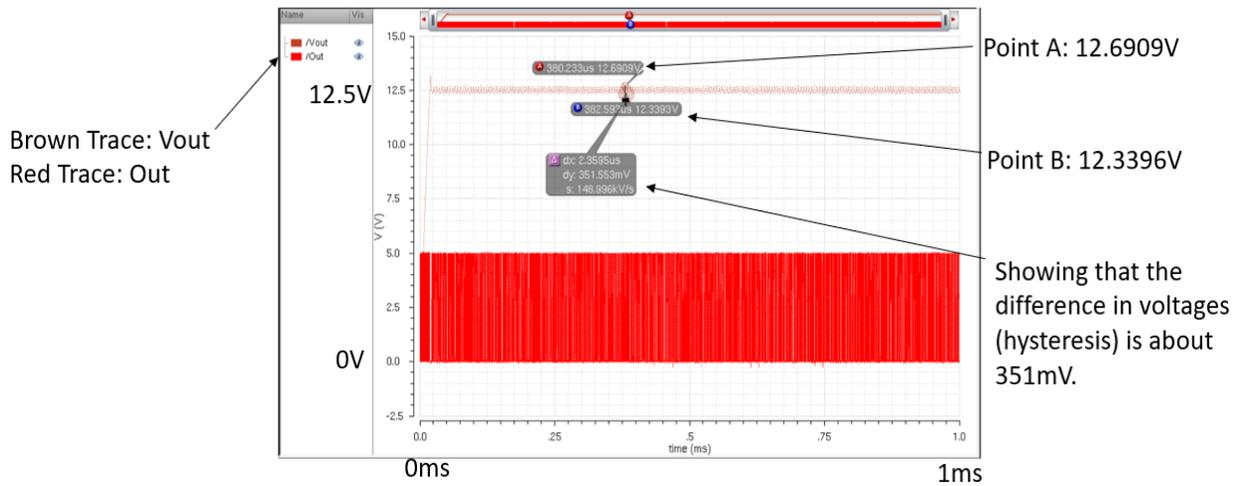
Figure 46 - Simulation Under Normal Conditions Showing Hysteresis
