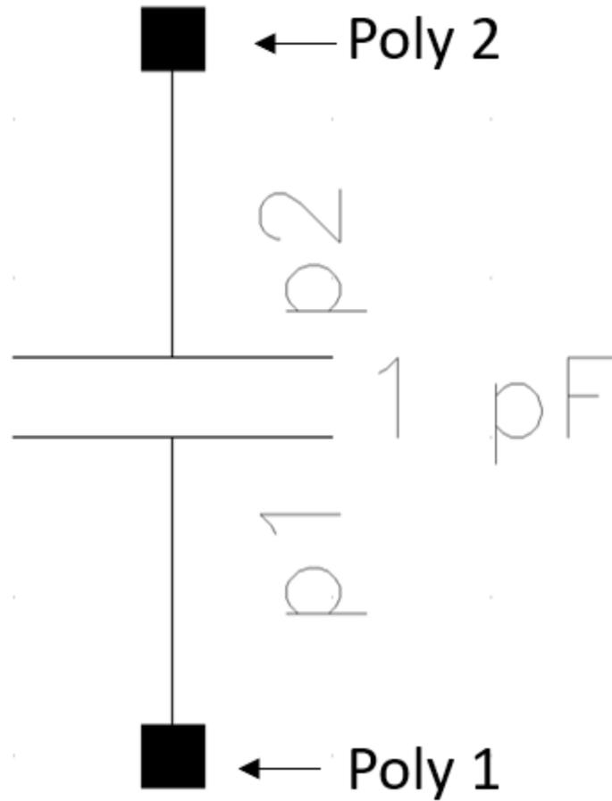
Figure 39 - 1pF Poly-Poly Capacitor Symbol
