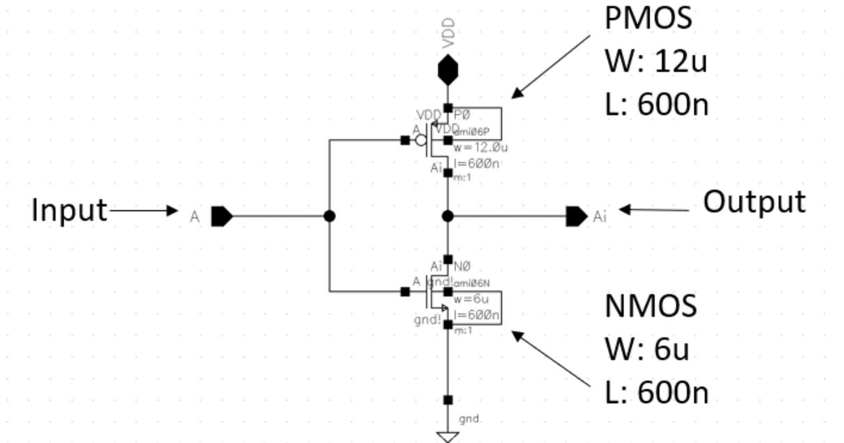
*Figure 21 - Inverter Schematic*
