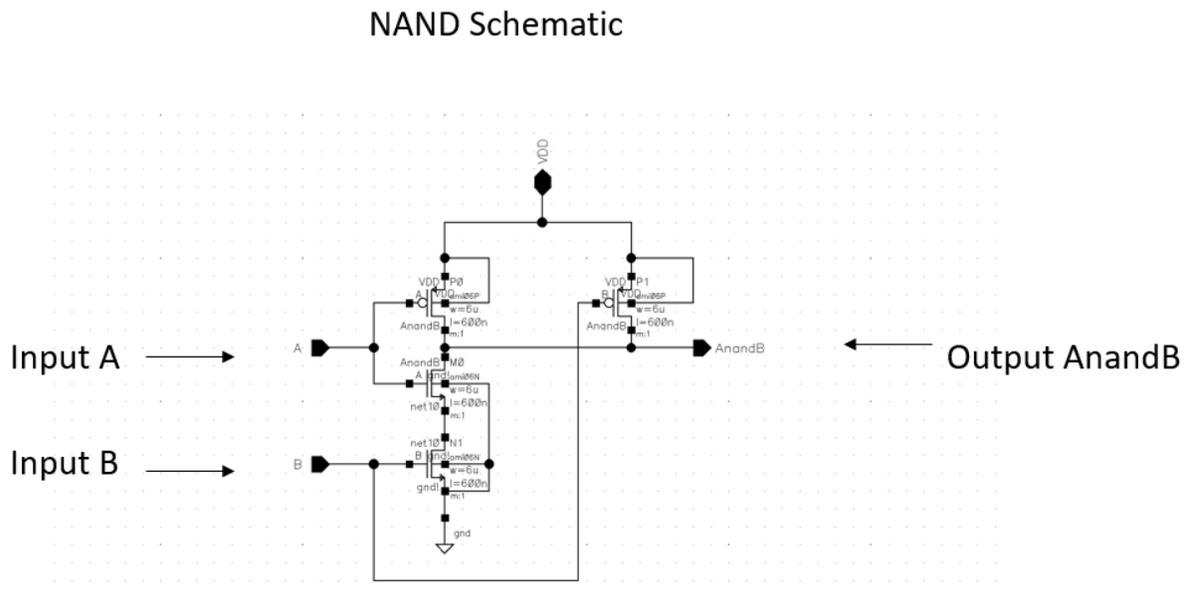
Figure 24 - NAND Schematic
