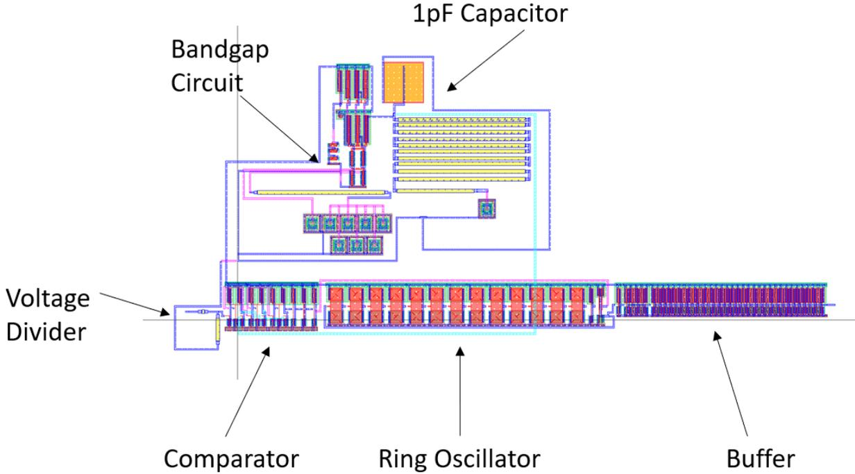
Figure 42 - Top Level Layout of the Controller Chip
