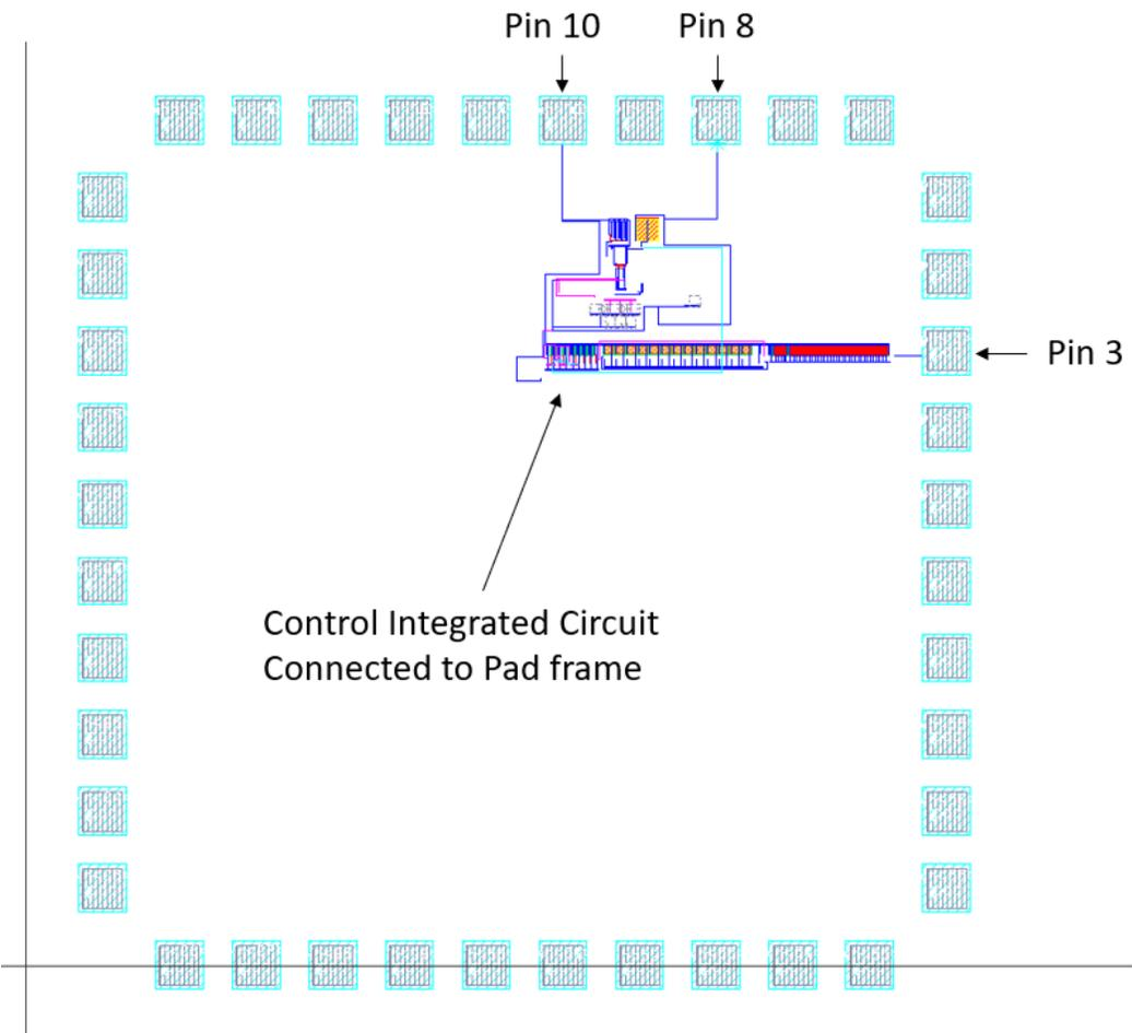
Figure 60 - Control IC Circuit Connected to Pad Frame
