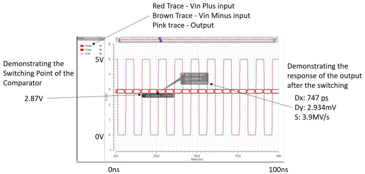
Figure 12 - Comparator Simulation
