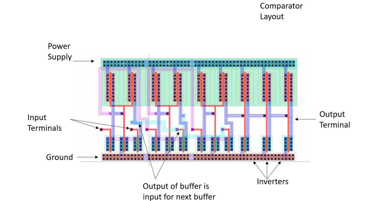
*Figure 10 - Comparator Layout*
