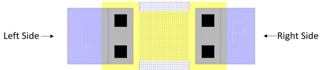
Figure 35 - 1k Hi-Res Resistor Layout
