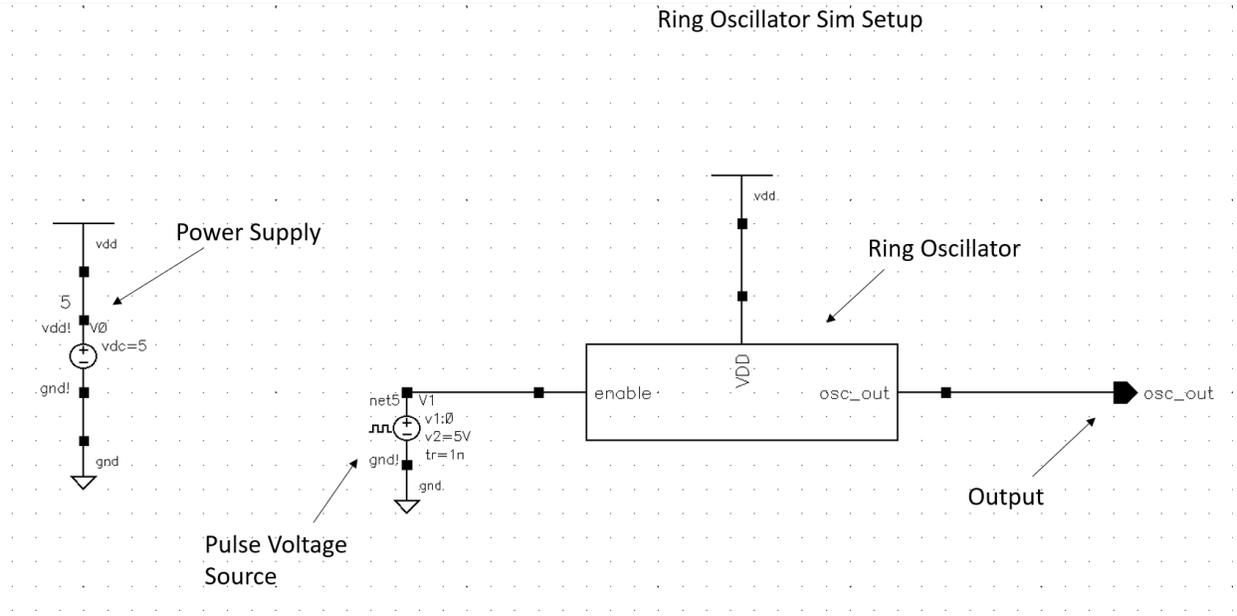
Figure 16 - Enabled Ring Oscillator Simulation Setup
