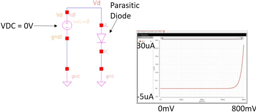
Figure 6 - Parasitic PNP Diode Response to Varying Diode Voltage
