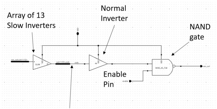
Output of slow inverters is the input of the normal inverter.
