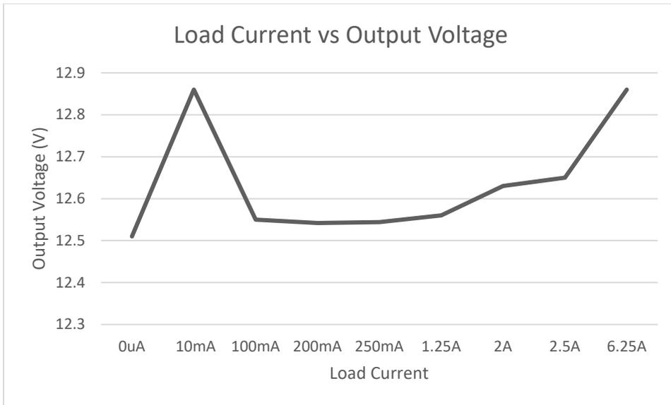
Figure 56 - Load Current Vs. Output Voltage
