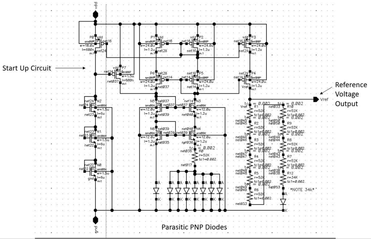
Figure 1 - Bandgap Schematic
