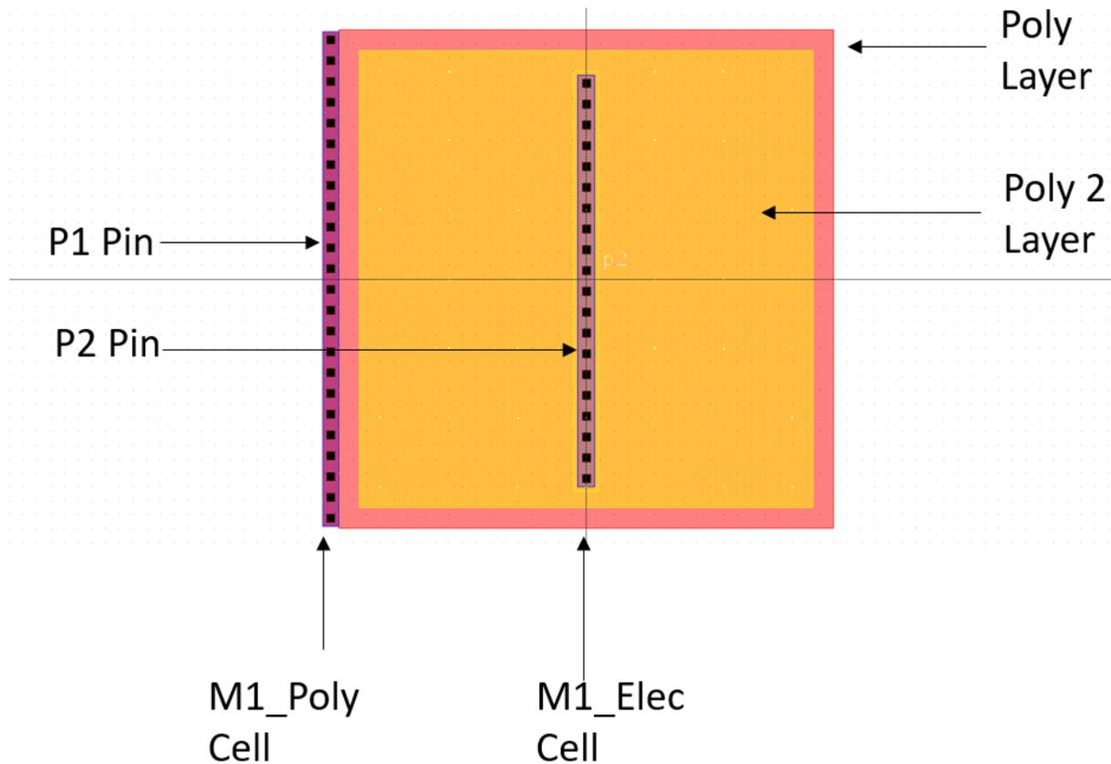
*Figure 40 - 1pF Poly-Poly Capacitor Layout*
