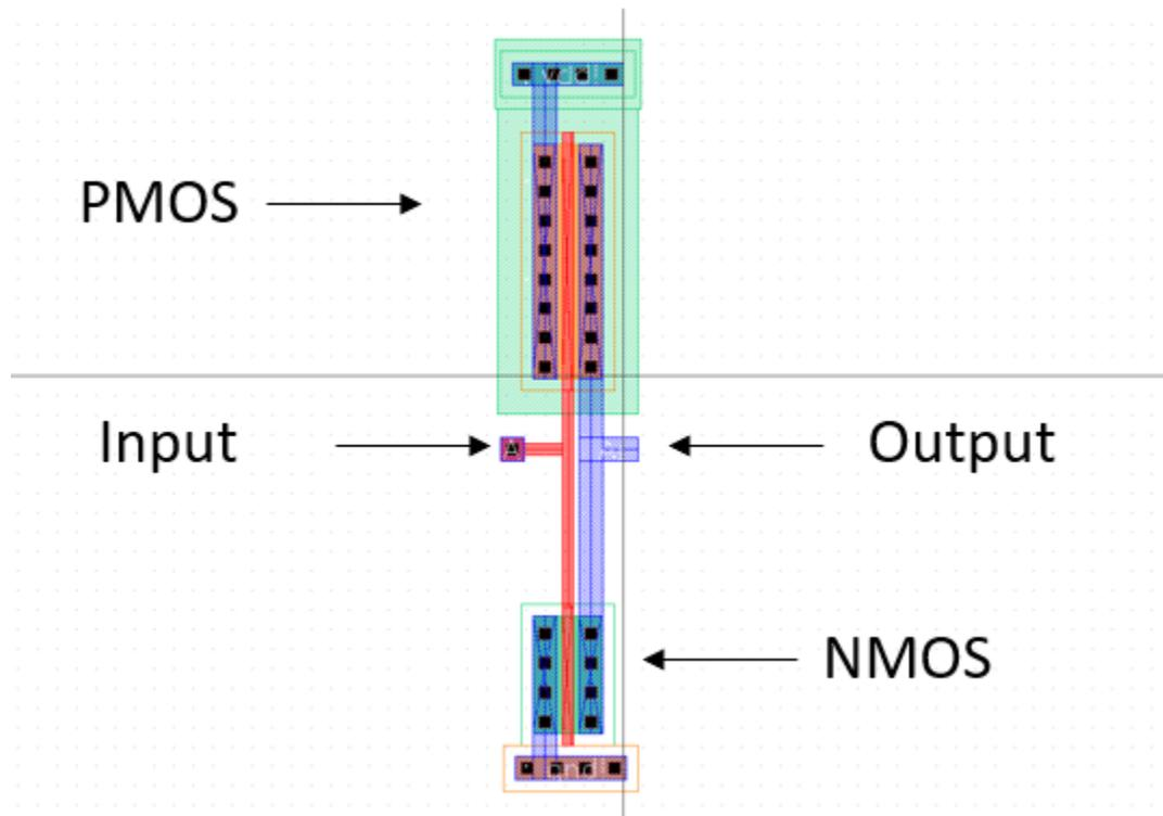
*Figure 23 - Inverter Layout*
