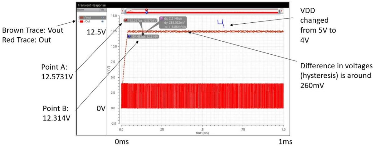
Figure 48 - Simulation where VDD is Lowered From 5V to 4V
