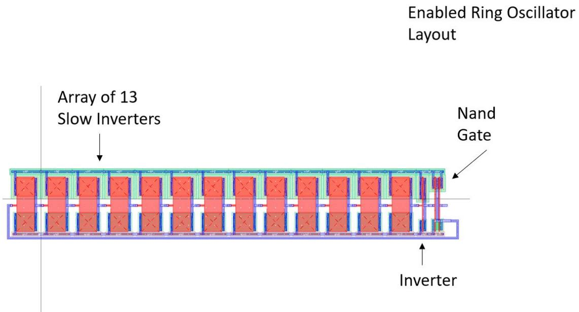
*Figure 15 - Ring Oscillator Layout*
