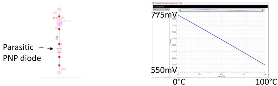
*Figure 7 - Parasitic PNP Diode Response to Varying Temperature*
