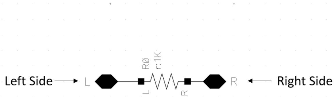
Figure 34 - 1k Hi-Res Resistor Schematic
