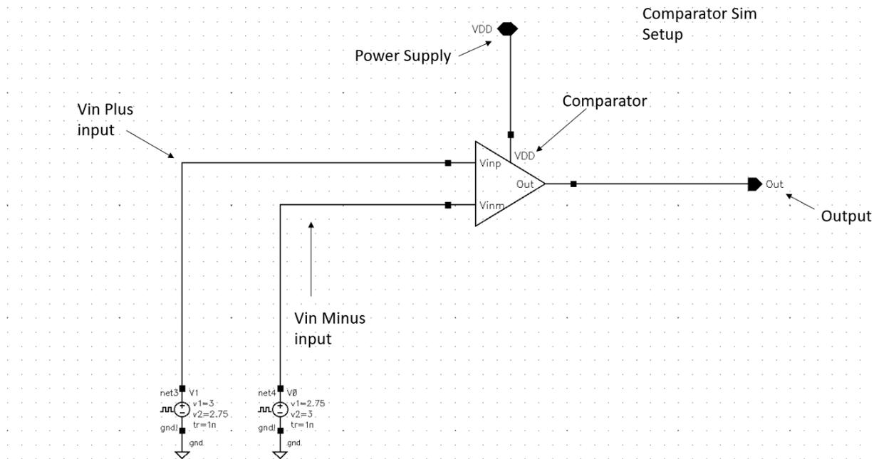
*Figure 11 - Comparator Simulation Setup*
