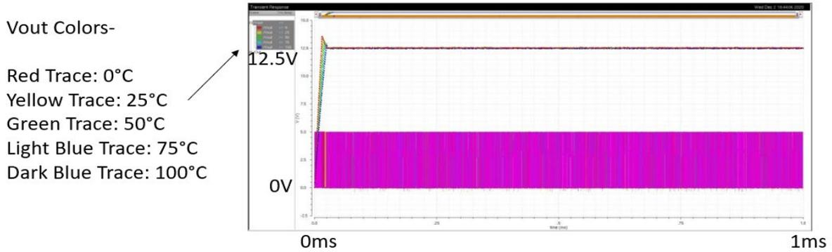
*Figure 47 - Simulation Run for Temperature Analysis*
