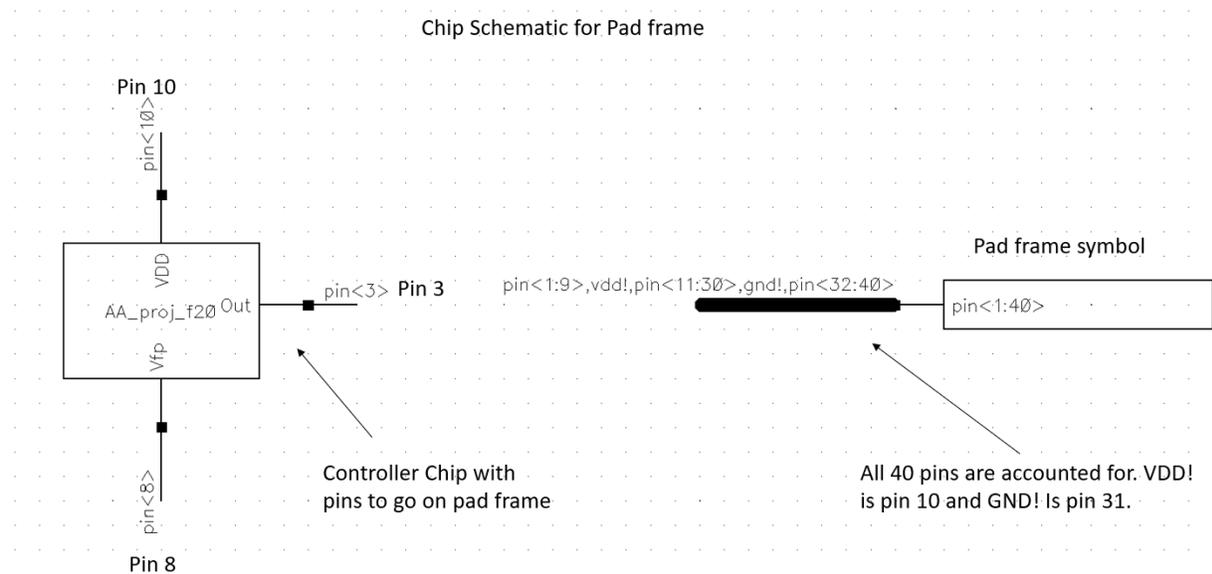
Figure 58 - Chip Schematic for Pad Frame
