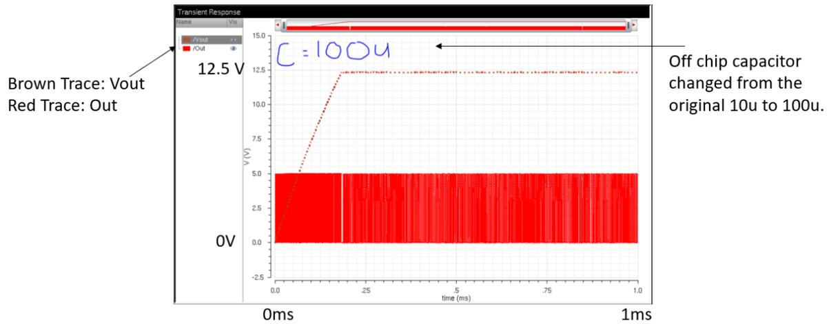
Figure 50 - Simulation with Different Off Chip Capacitor Value
