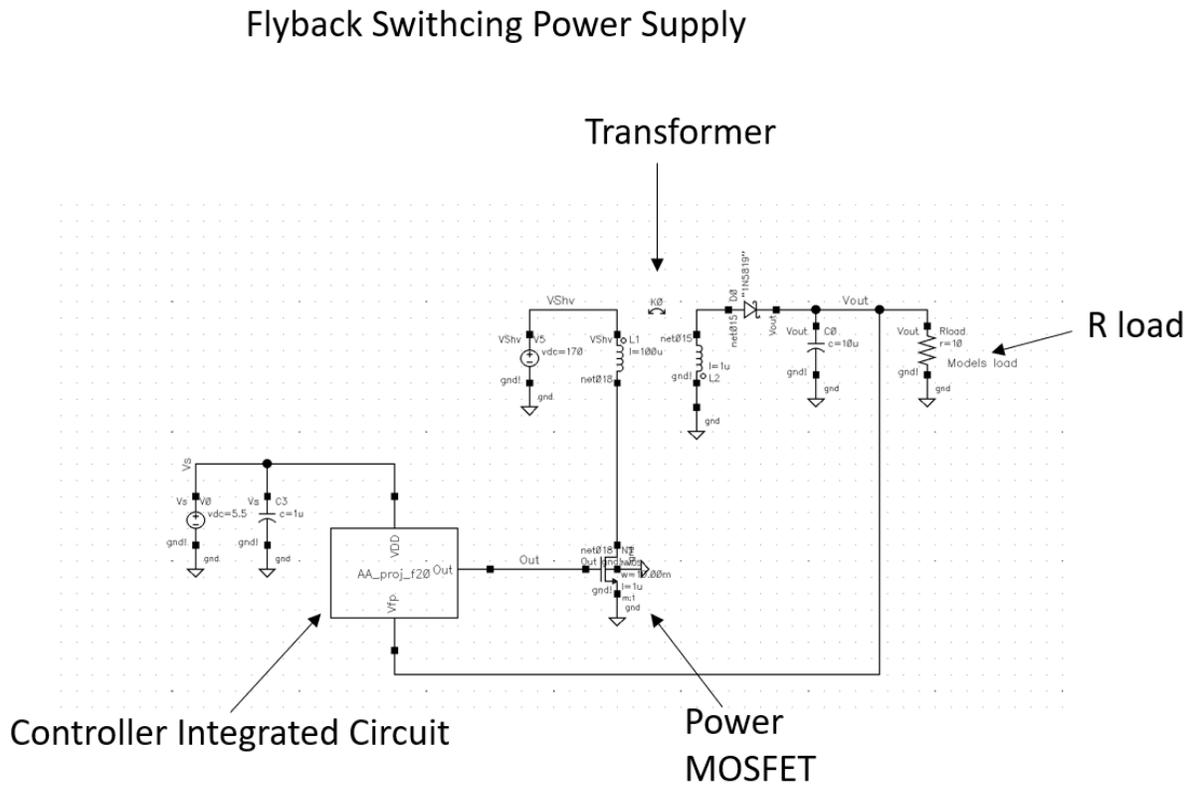
Figure 43 - Controller Chip with Off Chip Components for Flyback SPS
