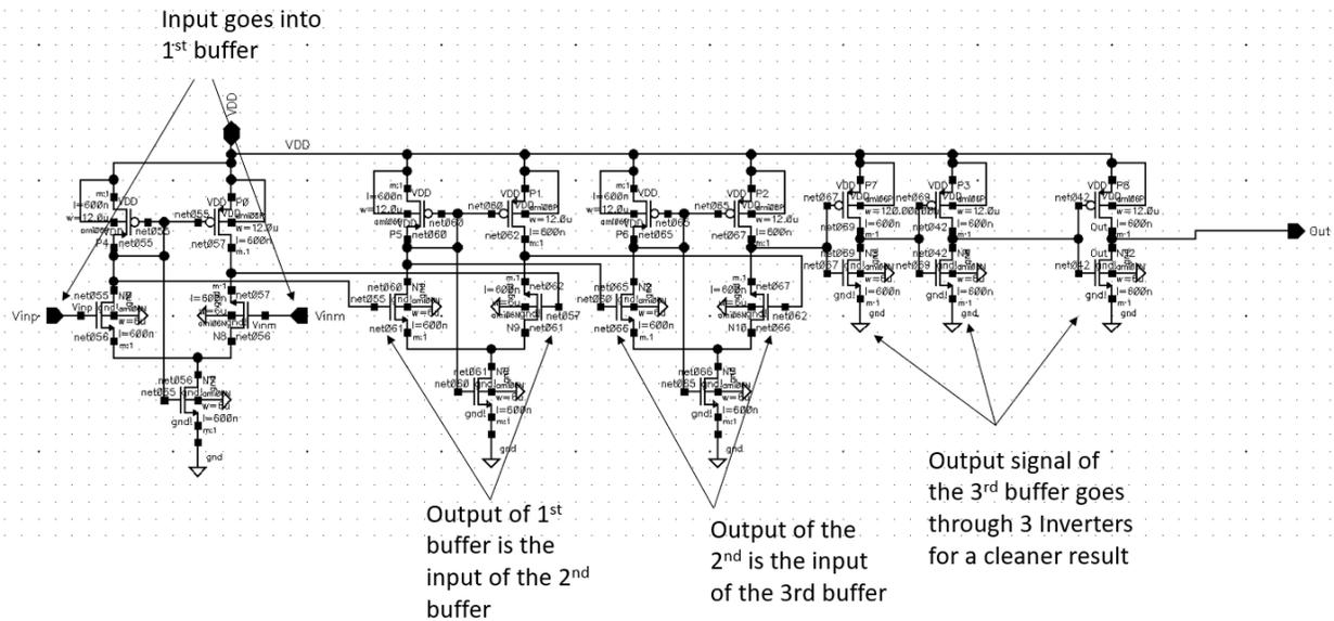
Figure 8 - Comparator Schematic
