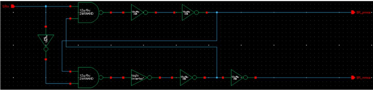
The reason for the inverter multiplier of 8 is to drive the PMOS and NMOS at the output.
