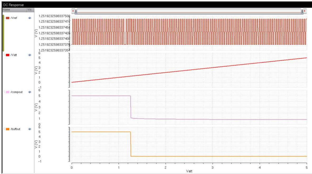
Now that I have my simulations I can find the gain of my comparator by taking the derivative of the output from the comparator. This will plot a line on the graph that will show me my gain at the point the output switches.
