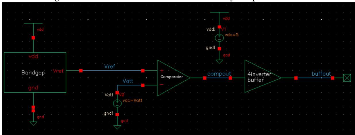
In this schematic I am using the bandgap circuit as my reference voltage and a dc voltage source as my  $V_{out}$ . I will sweep the voltage on the source to simulate the output voltage oscillating around 2.5V.
