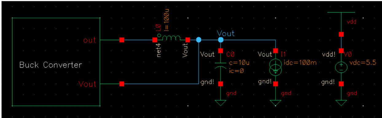
Simulation of the power supply using a pulsed current source to simulate a load:
