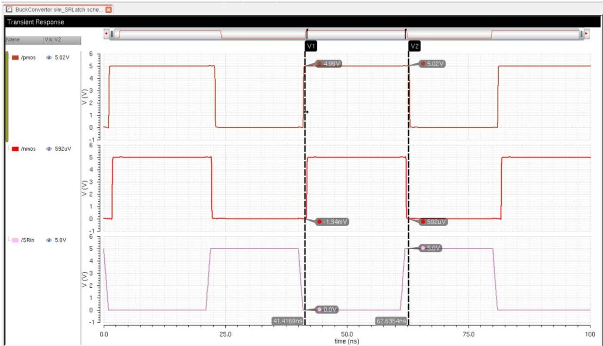
We can see that the PMOS turns off before the NMOS turns on. This helps improve the efficiency of the circuit since we won't be shorting the source to ground. This is accomplished by having a big enough time delay from the NAND gates and the inverters.
