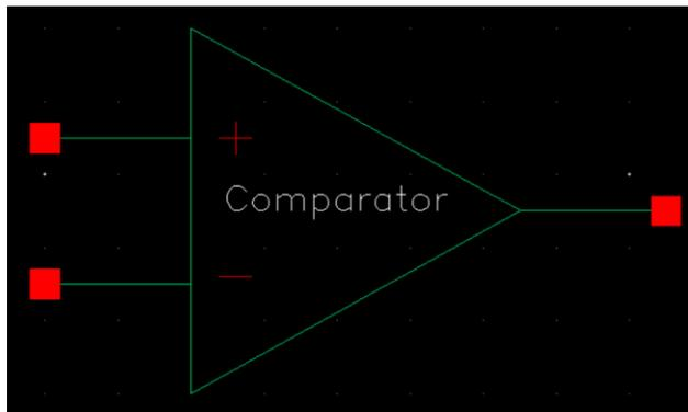
The implementation of this circuit in my overall design will be used to compare the output voltage with the bandgap voltage and dictate whether the PMOS or the NMOS should be on. Since the bandgap reference voltage is at 1.25V and our desired output voltage is 2.5V we will need to have our output voltage go through a voltage divider before entering our comparator.
