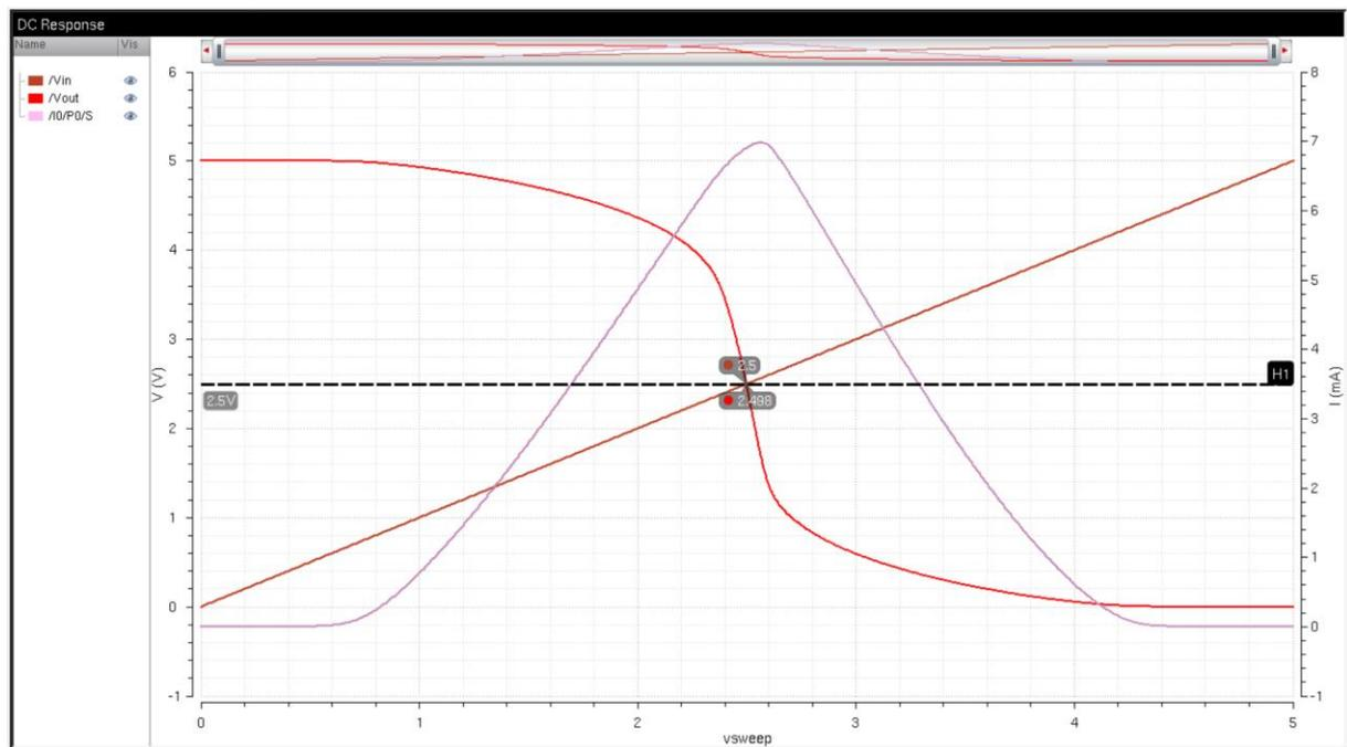
We can see that the switching point of my inverter is at 2.5V. This is because the width of my PMOS is twice the width of my NMOS. We can also see that the only time current will flow is during the change from 5V to 0V.
