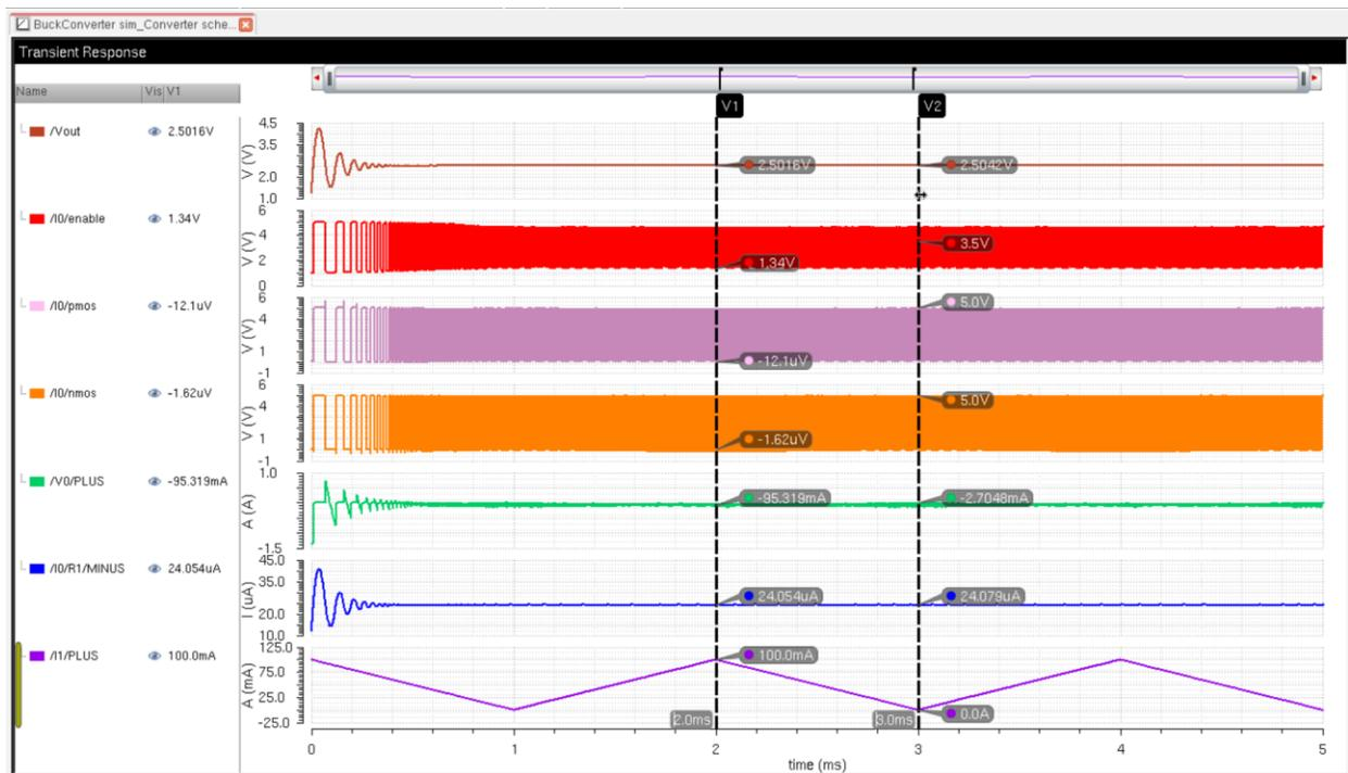
The output voltage is at a 2.5V with very small oscillations around 2.50X. These oscillations are from the comparator turning the PMOS and NMOS on and off. Although the current is changing the output voltage stays a constant 2.5V.
