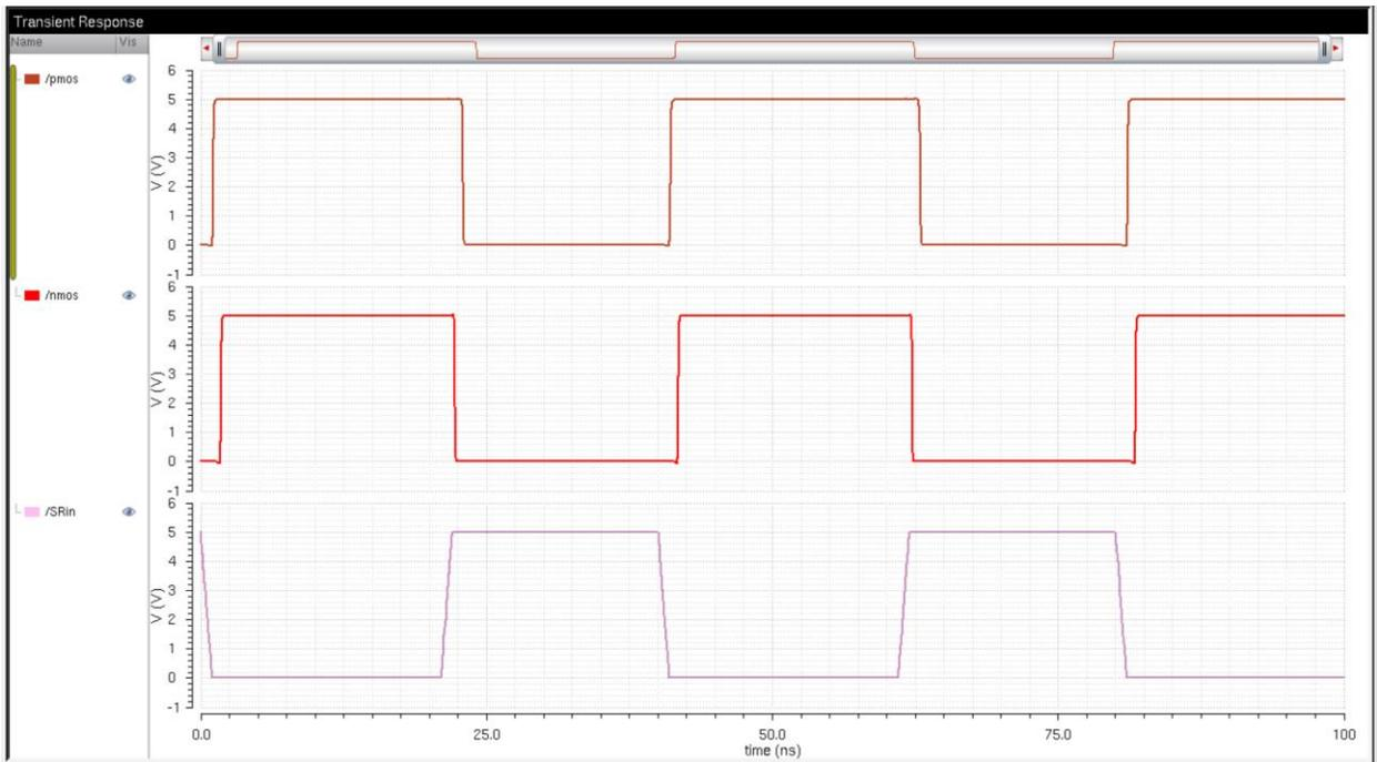
We can see that both outputs are at the same logic. This is because we want the PMOS and NMOS to be enabled at different times. This is to eliminate cross-over current and improve efficiency.
