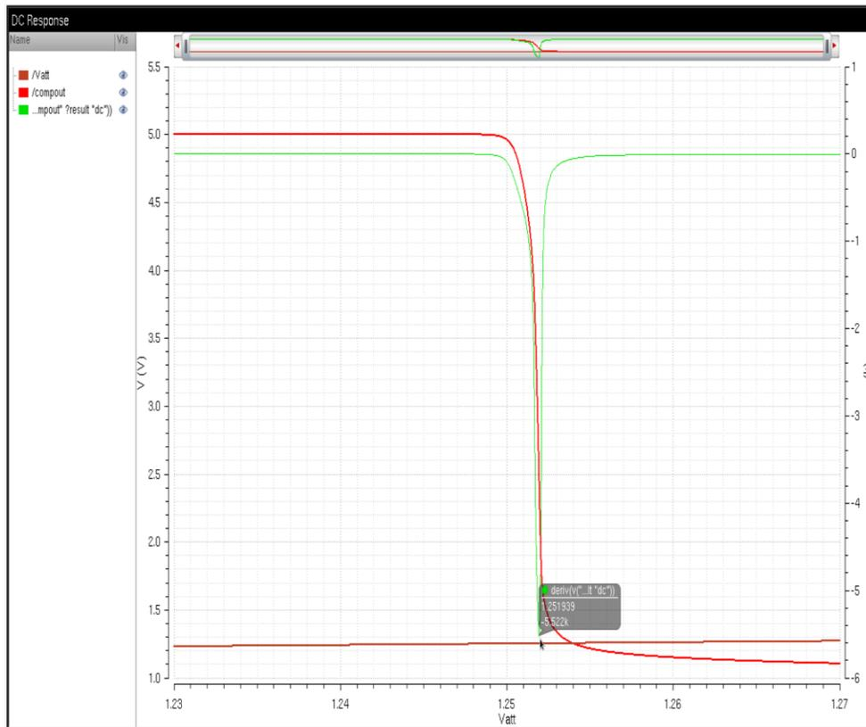
In this simulation, we can see that the gain is a negative number. This is because the output voltage is going from high to low giving us a negative slope. The maximum magnitude of this line is the gain of the comparator.
