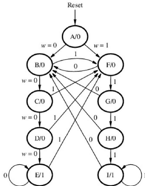
Figure 2. A state diagram for the FSM.
