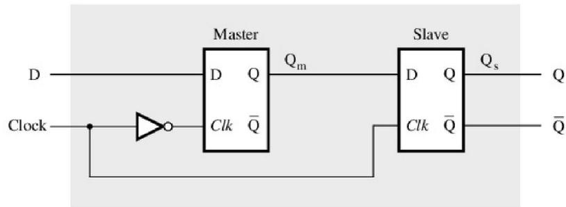
Figure 5. Circuit for a master-slave D flip-flop.
