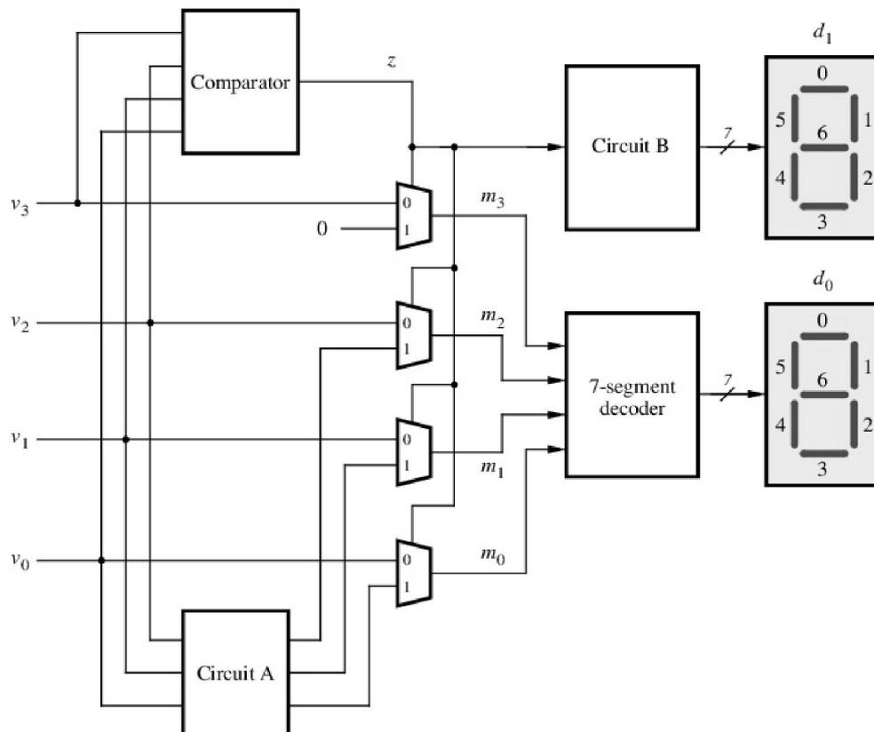
Figure 1. Partial design of the binary-to-decimal conversion circuit.
