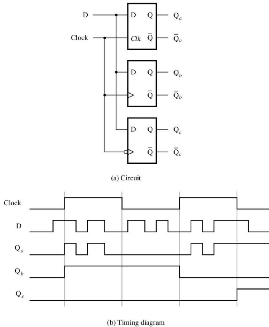
Figure 6. Circuit and waveforms for Part IV.
