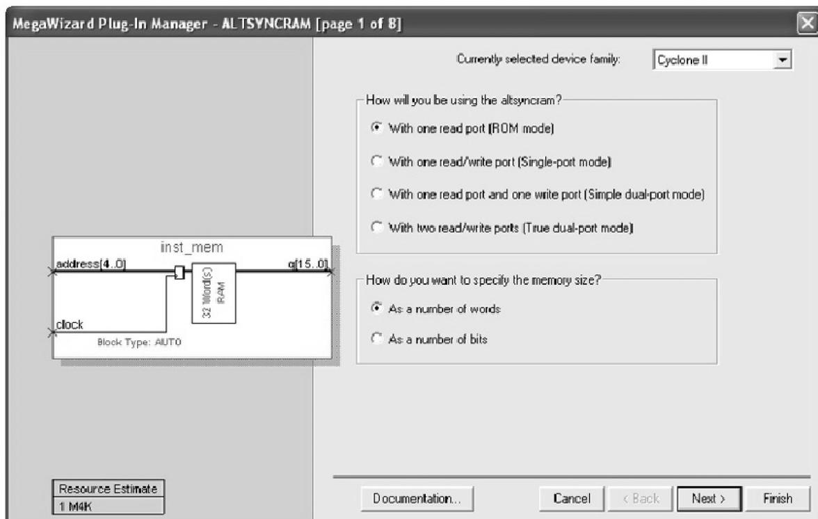
Figure 5. ALTSYNCRAM configuration.
