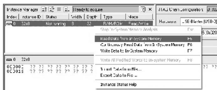
Figure 10. Using the In-System Memory Content Editor tool.
