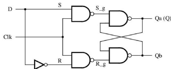
Figure 4. Circuit for a gated D latch.
